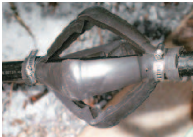
Figure 8. This two-piece torque arrestor prevents the motor from chafing the wires as the pump turns on and off.
