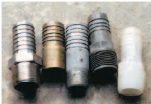
Figure 7. The two fittings on the left are the only ones you want to use. The others are guaranteed to break, crack, and split.
