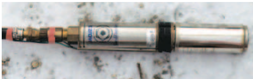
Figure 6. The lower part of the pump houses the motor, and the top half contains the pumping mechanism (the pump head). The plastic section between the two is the inlet for the water. The wires are secured to prevent chafing.
