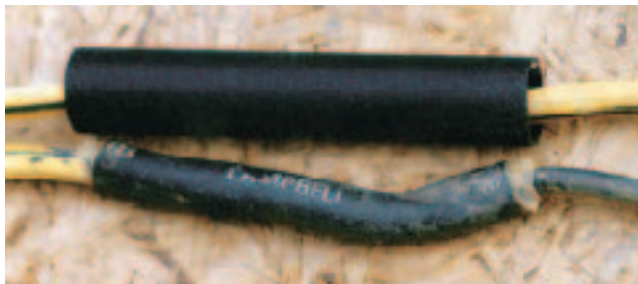
Figure 5. A submersible splice kit connects the pump motor to the submersible pump wire running to the wellhead (top). In the photo below, the shrink tube on the top has not been heated. The bottom wire shows how the tubing shrinks to form a watertight seal.
