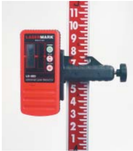
Figure 1. The best detectors have a beeping tone that changes to a steady tone when the beam is on the mark.
