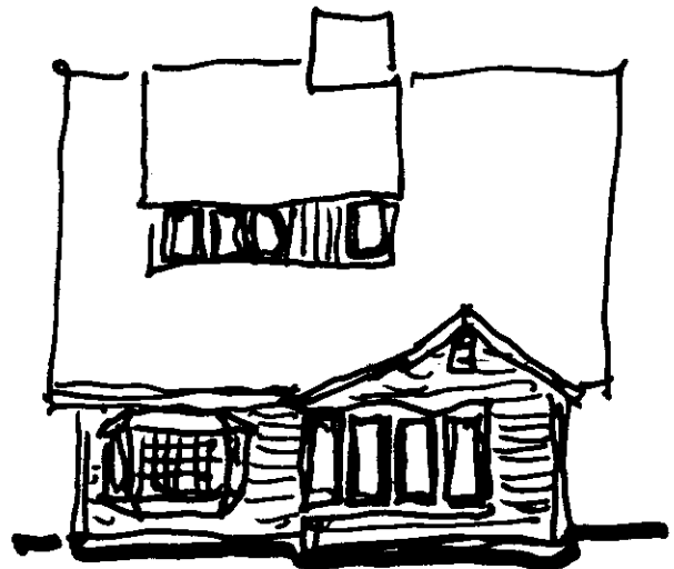
Figure 2. The historically authentic rear elevation of the same saltbox-style house, on the other hand, is poorly adapted to modern lifestyles (left). Today’s version is more likely to look like the drawing at right. The increased glass area makes for a brighter interior, but laying out windows around appliances, closets, and other obstructions results in an awkward-looking, unbalanced elevation.
