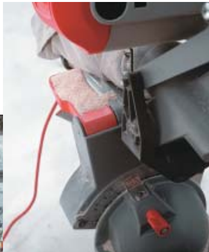
Figure 1. The MS1290's bevel lock (covered with sawdust in photo above) is located right up front, so you don't have to reach around the back of the saw to make adjustments.
