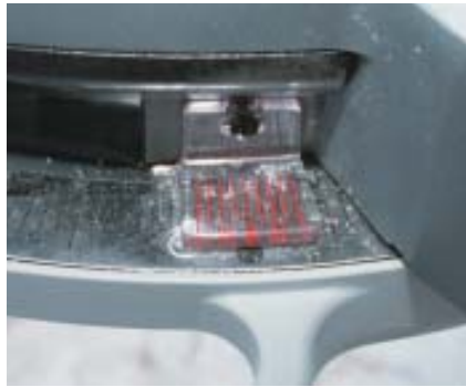
Figure 3. Laser-etched numbers provide good contrast on the miter scale; indicators are adjustable to help maintain accuracy (left). Settings for cutting crown on the flat are included on the miter scale, but they only work for crown with a 38° spring angle (right).
