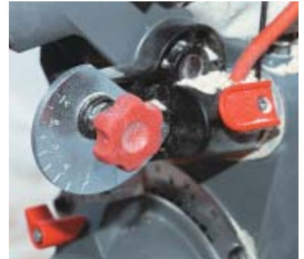
Figure 4. The depth stop, which also serves to lock the cutting head for transport, is the weak link in the MS1290's otherwise excellent set of controls. Rotating the cam stops the blade at the desired depth, but fine-tuning the setting is more difficult than with a typical threaded stop.
