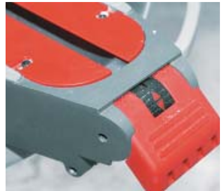
Figure 2. Instead of a spring-loaded lever, a thumbwheel controls the stops for common miters, and a fast-adjusting lever locks the miter table. Raising the lever releases the table; pushing it down locks it securely.
