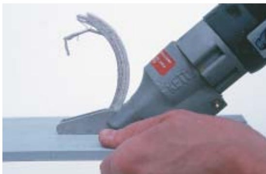
Figure 1. With a cutting action similar to that of scissors, shears crush the material between hardened steel blades. Replacement blades cost about $65, and makers claim that the blades will last for about five 2,000-square-foot houses.
