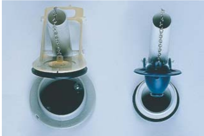
Figure 2. The 2-inch flapper valve at right has long been the industry standard. A new 3-inch valve recently introduced by Toto (left) empties the tank faster and provides an aggressive flush with little swirling in the bowl.
