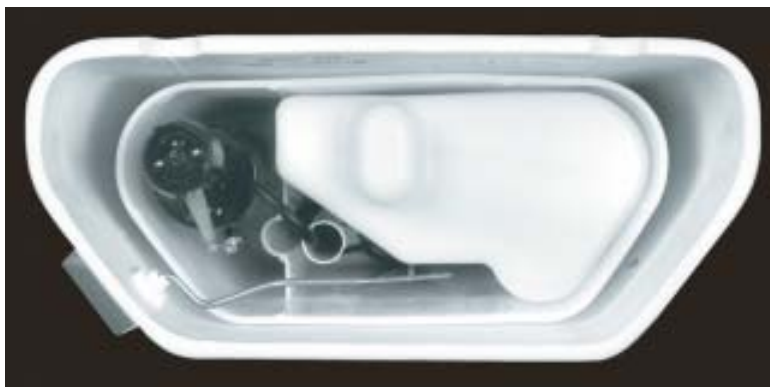
Figure 4. The outwardly conventional-looking Briggs Vacuity (top) develops increased flushing force with an internal tank-mounted vacuum-assist unit (above). As water drains from the closed unit during the flush cycle, an internal connecting tube induces a partial vacuum in the upper portion of the trapway.
