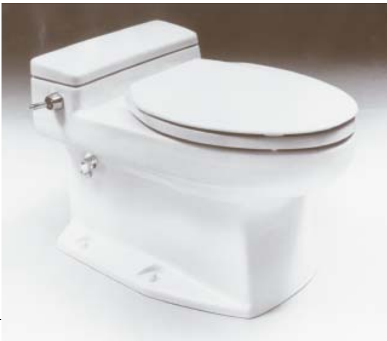
Figure 6. Microphor makes two residential toilets that use a mere 2 quarts per flush. While the need for a separate source of compressed air makes this impractical for most applications, it's a useful option where local water restrictions or a low-yield well rule out conventional low-flow fixtures.
