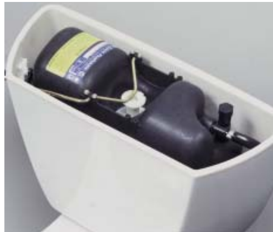
Figure 3. Pressure-assisted toilets use air trapped in a sealed vessel to deliver a forceful — and noisy — flush. Although pressure-assisted fixtures are outwardly similar to conventional gravity toilets, bowl and trapway designs differ. As a result, existing gravity fixtures can't be adapted to work with a pressure-assisted unit.
