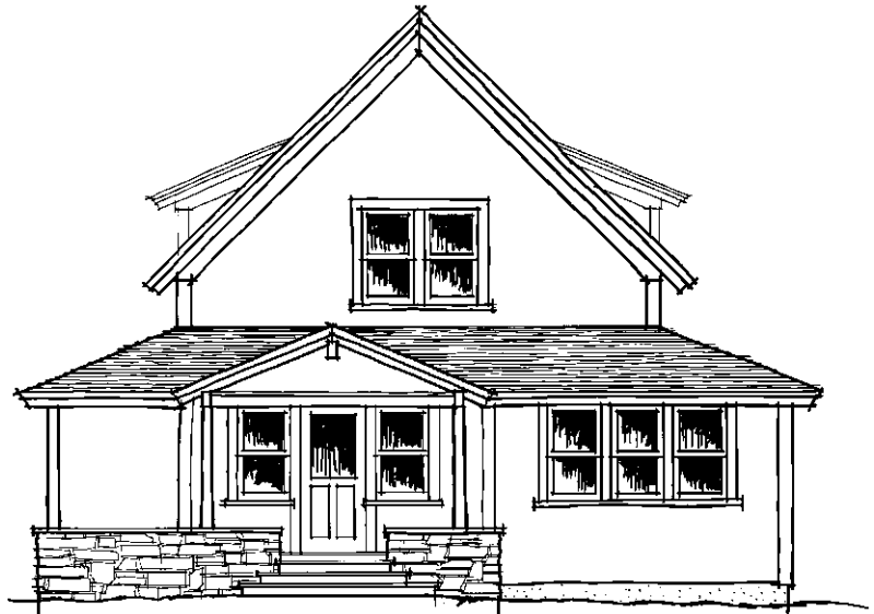
Figure 4. The stripped-down gable elevation above is improved by the addition of a wraparound porch and low-pitched dormers (right). The broader base also helps tie the house to the ground and provides a sheltering entryway.
