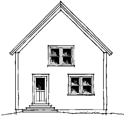
Figure 4. The stripped-down gable elevation above is improved by the addition of a wraparound porch and low-pitched dormers (right). The broader base also helps tie the house to the ground and provides a sheltering entryway.
