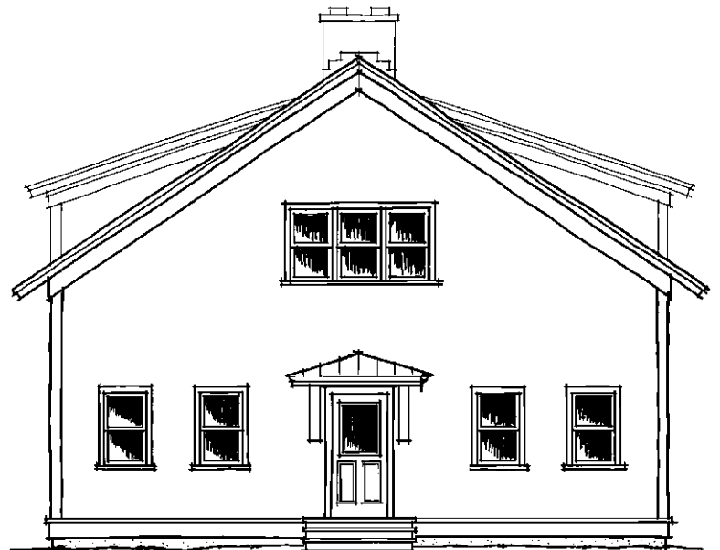
Figure 3. A two-story plan is a fine way to enclose a maximum amount of space at minimal cost, but without skillful detailing, the gable end often presents an awkward, top-heavy look (above). Lowering the roofline is a simple way to provide a better-proportioned facade, although it complicates the framing and interior finish. Shed dormers can be added if additional space is needed upstairs (right).
