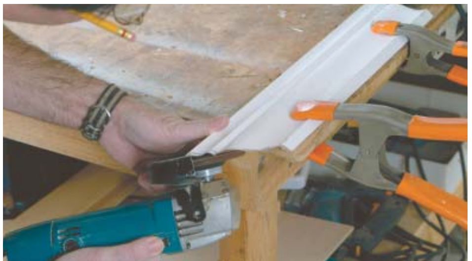
Figure 2. To cut the unusual scribes that are required when fudging an inside corner (above), the author uses a jigsaw fitted with a coping foot (above right), as well as a grinder (right), for making extra steep back bevels.
