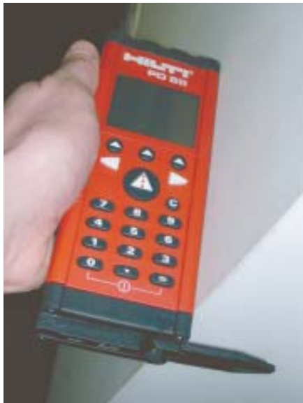
Figure 1. Measuring from an outside corner or locating a window is easier with a hook for outside measurements. The Trimble Spectra HD150's computer automatically compensates for length when you attach the hook (left). The Hilti PD22 and PD28 use a foldout hook for outside corners (right).
