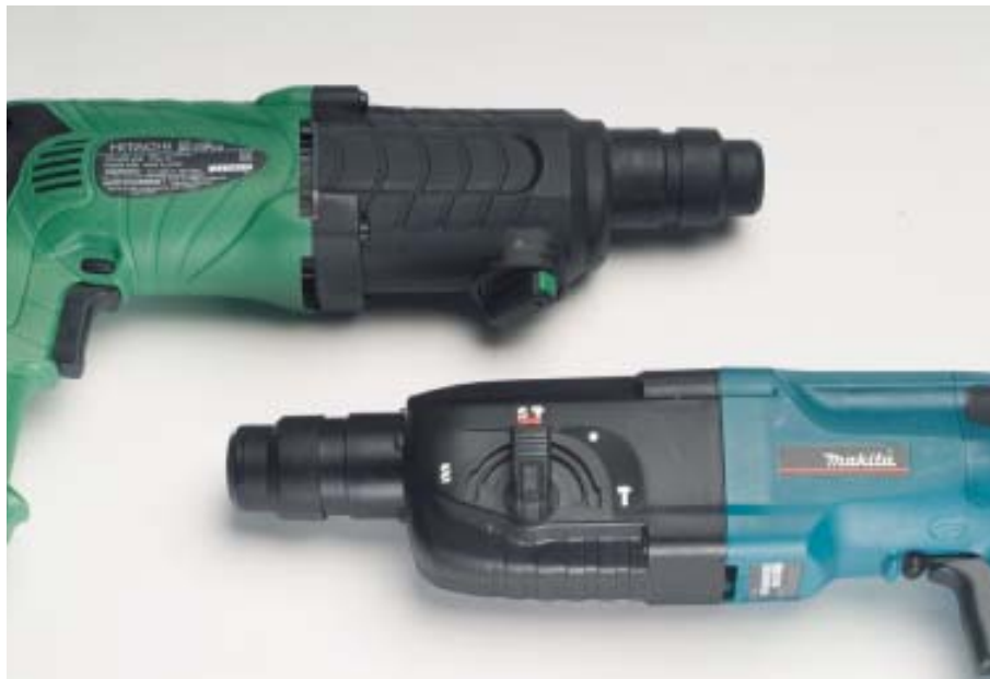
The Hitachi (top) and the Makita have different selector switches, but both are easy to engage.
