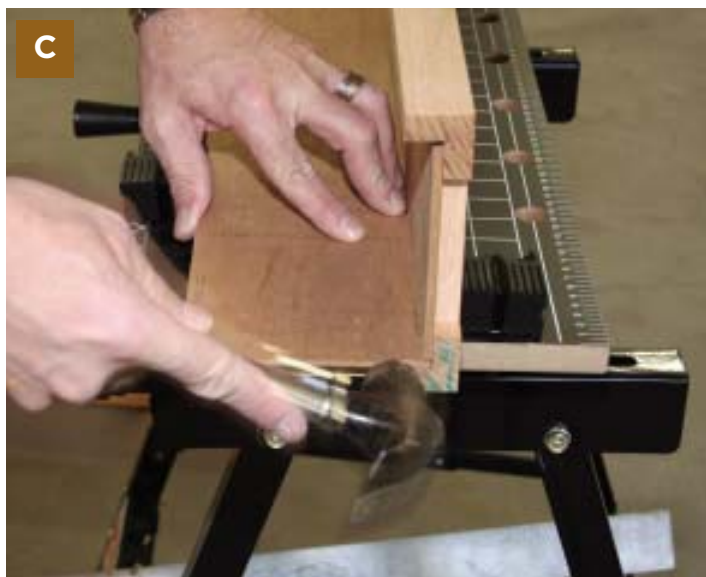
Figure 2. To make the panels, oak cross rails are glued on the front (A) and pinned from the back (B). The finished panel is then tapped into place in the slot left by the spacer (C). Construction adhesive and brads secure it (D).
