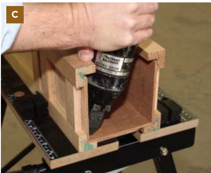
Figure 3. The third panel, with corner frame attached, is slipped over the second plywood panel (A) and glued and pinned (B, C).
