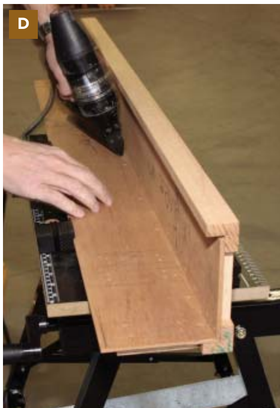
Figure 2. To make the panels, oak cross rails are glued on the front (A) and pinned from the back (B). The finished panel is then tapped into place in the slot left by the spacer (C). Construction adhesive and brads secure it (D).
