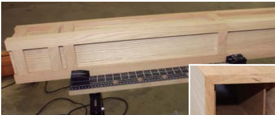
Figure 5. The newel is finished with a 12-inch-wide oak base, then capped and trimmed on site.
