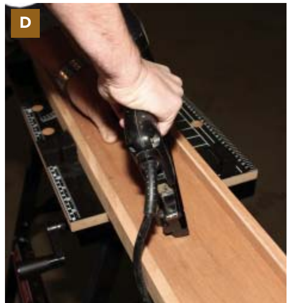
Figure 1. Newel construction starts with four 2x2 oak balusters with one corner ripped out. Plywood panels are glued with PL400 (A), then pinned in place (B). By using a plywood spacer while nailing the first panel to the second baluster (C, D), the author leaves room for the next perpendicular panel to slip snugly into place.
