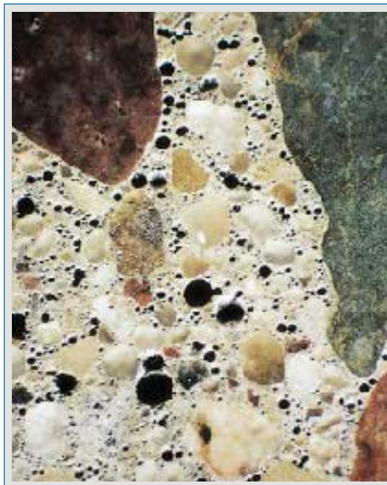
Figure 4. In this magnified slice of air-entrained concrete, the separated air bubbles provide space to relieve the pressure of expanding ice. Air-entrained concrete surfaces will endure many years of winter freezing and thawing.
