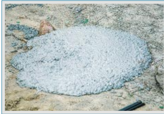
Figure 7. Stiff, low-water-content concrete (left) is easy to tell apart from concrete with a lot of added water (right). Slump tests (below) are used on site to maintain uniform water content in successive loads of the same mix. The 9-inch to 10-inch slump shown by this example (measured from the height of the cone to the top of the slumped concrete) is not as hard to work with as a stiffer mix, but may contain too much water. To increase slumps without adding water, consider a superplasticizing admixture.
