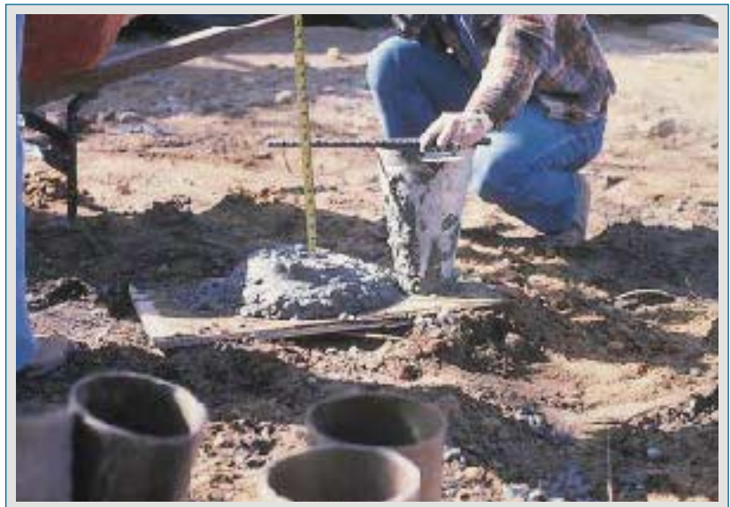
Figure 7. Stiff, low-water-content concrete (left) is easy to tell apart from concrete with a lot of added water (right). Slump tests (below) are used on site to maintain uniform water content in successive loads of the same mix. The 9-inch to 10-inch slump shown by this example (measured from the height of the cone to the top of the slumped concrete) is not as hard to work with as a stiffer mix, but may contain too much water. To increase slumps without adding water, consider a superplasticizing admixture.
