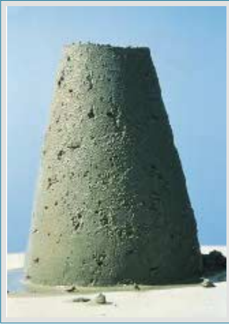
Figure 7. Stiff, low-water-content concrete (left) is easy to tell apart from concrete with a lot of added water (right). Slump tests (below) are used on site to maintain uniform water content in successive loads of the same mix. The 9-inch to 10-inch slump shown by this example (measured from the height of the cone to the top of the slumped concrete) is not as hard to work with as a stiffer mix, but may contain too much water. To increase slumps without adding water, consider a superplasticizing admixture.
