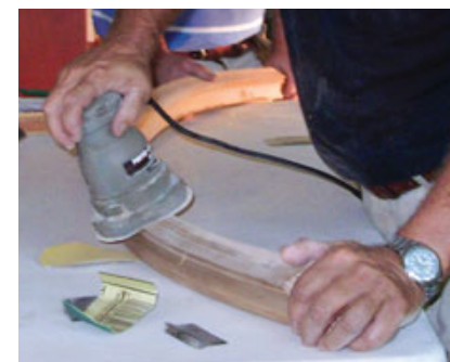
Figure 3. To minimize springback, rail sections should set at least 72 hours before they're removed from the form (left). Cleanup is done with scrapers, sanders, and Tadpole profiled sandpaper holders for the beads and hollows (below).
