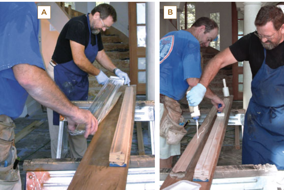
Figure 1. The author lines the bending mold with shrink-wrap to keep glue from sticking to the rail and bending mold (A). After applying an even coat of glue to each lamination with a 2-inch roller (B), the author lightly mists the glue with water (C). A few quick wraps with plastic at the ends and in the middle secures the bundle (D).
