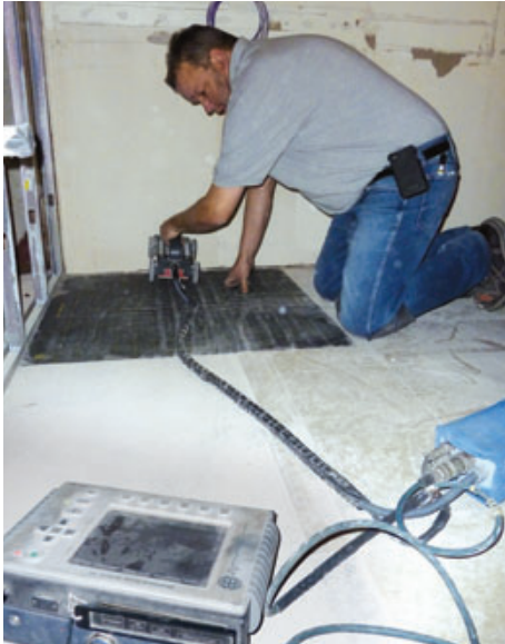
Figure 1. A technician uses ground-penetrating radar to map the position of electrical conduits and other obstructions in the reinforced slab floor (above left). Unlike a wheeled scanner, his handheld scanner can't map results or plot exact depths, but it can get closer to walls (above right).
