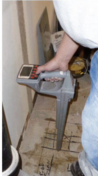
Figure 1. A technician uses ground-penetrating radar to map the position of electrical conduits and other obstructions in the reinforced slab floor (above left). Unlike a wheeled scanner, his handheld scanner can't map results or plot exact depths, but it can get closer to walls (above right).
