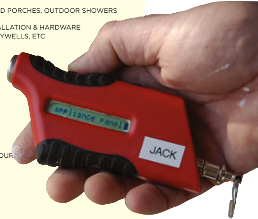
Figure 2. The author programs his employees' red FastTrakkers with simplified cost codes and job descriptions (A), which are also printed out and displayed on site. These simplified codes correspond to CSI MasterFormat cost codes (B), which the author uses for estimating and job-costing.
