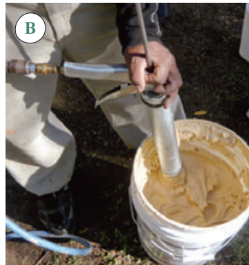
Figure 1. Depending on the situation, air-sealing can call for caulk, canned foam, tape, sheet material, or a combination of materials. The author's job-site arsenal covers all the bases (A). High-performance bulk caulk, applied with refillable pneumatic caulking guns, is a useful alternative to canned foam for many applications (B). If air-sealing is going to be done right, someone has to sweat the details. The author's shirt leaves no doubt as to who that person is (C).
