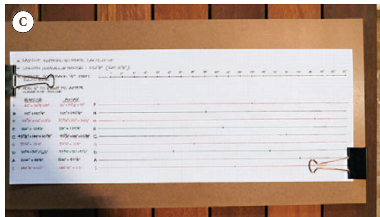
Figure 3. The author set up the cut station in his shop (A) parallel to a layout bench where he transferred the layout marks from the story poles to the decking (B) for crosscutting and predrilling. He followed a color-coded chart (C) to ensure the courses were cut and labeled accurately for installation in the field.
