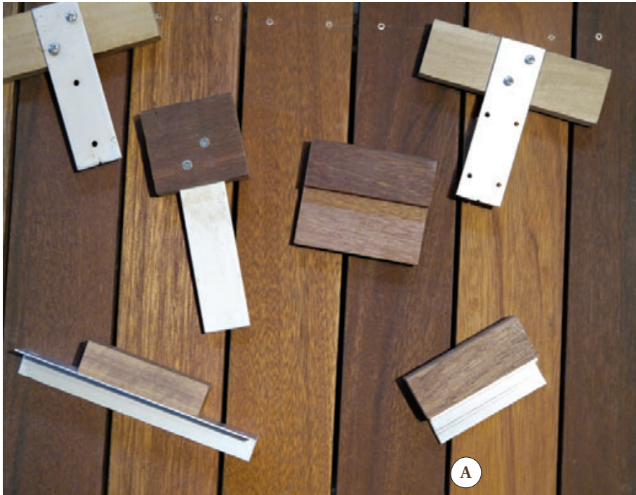
Figure 5. Jigs made with hardwood scraps and aluminum stock (A) sped up accurate drilling and spacing of deck boards. In combination with the use of a BoWrench, the spacers ensured near perfect spacing (B,C).
