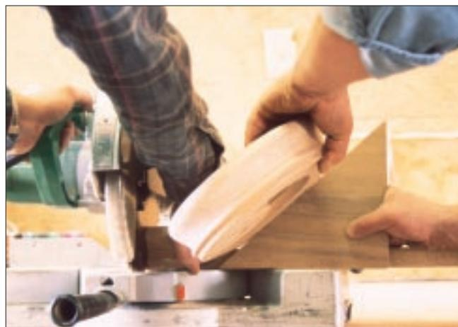
**Figure 7.** The pitch block can be used as an angle guide when cutting curved easements. The miter saw remains set at 90 degrees.
