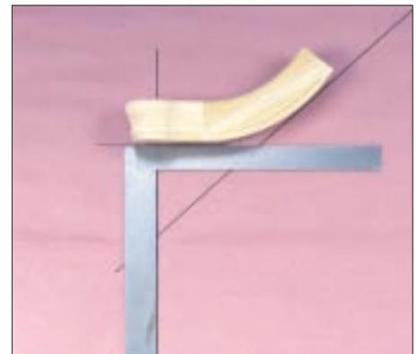
**Figure 4.** To find the height of the starting newel, center the dowel hole in the starting easement over the newel centerline. Using a framing square to keep the easement level, slide the easement down until its curved underside touches the rail layout line. Make a horizontal mark where the pin hole intersects the newel centerline to establish the newel post height.
