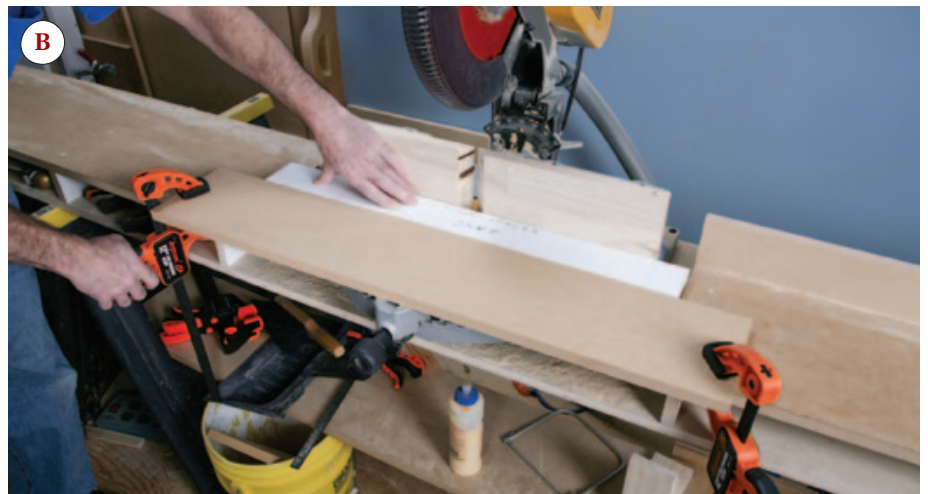
Figure 2. With the crown upside-down, the author measures its horizontal projection (A), then rips a gauge block that width to use in setting the crown stop (B).
