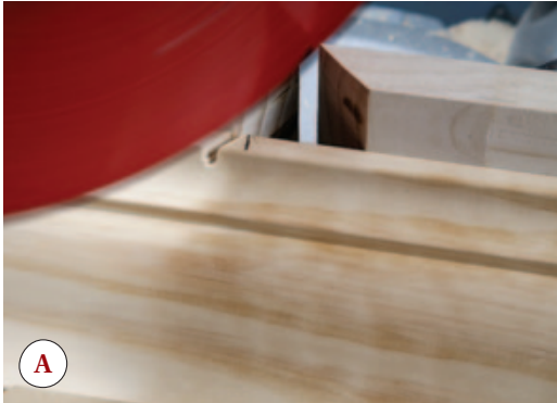
Figure 3. To use the “creep method” for cutting crown, make a shallow cut close to the line (A), then — with the material firmly pressed between your thumb and the fence — slide it into position for the final cut (B).
