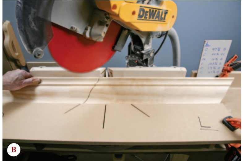
Figure 3. To use the “creep method” for cutting crown, make a shallow cut close to the line (A), then — with the material firmly pressed between your thumb and the fence — slide it into position for the final cut (B).
