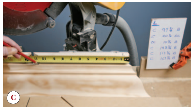
Figure 4. After measuring and cutting a coped end to length (A), the author cuts off the tip before removing the piece from the saw (B). When cutting outside corners (C), he pulls the measurement from the auxiliary fence, with the short point of the miter flush with the fence.
