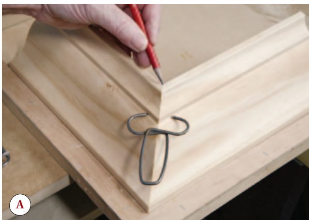
Figure 8. Using a corner mockup (A) to lay out outside corners (B) saves time when cutting the joints.
