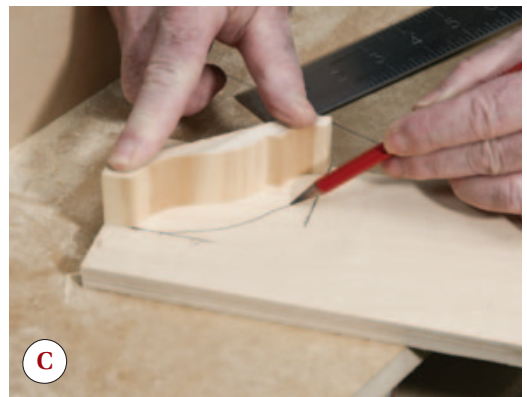
Figure 6. A crown holder (A) positions the molding for precise installation, and is also an ideal layout tool (B). It's simple to make from a scrap of plywood (C).
