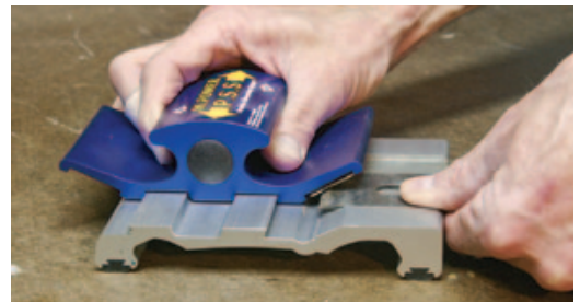
To sharpen a plane blade or chisel with the PSS1, you simply place it on the base and run a diamond stone housed in the carriage back and forth over it.
