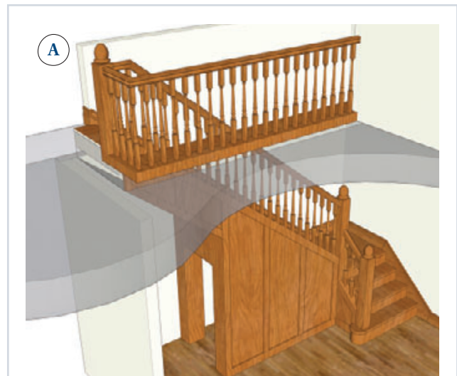
Figure 3. Once the first and last balusters of this stair rail were positioned, SketchUp could be instructed to add a selected number of evenly spaced balusters between them. A couple of tries were needed to come up with a spacing that complied with the stair code (A). The final version also reflects a change to the handrail-to-newel post connection, made when the client rejected the gooseneck connection in an earlier drawing (B).
