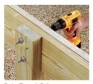
Faster Through-Bolt. If you're still using a socket wrench to fasten posts or beams, you might want to check out the *ThruLok Screw Bolt Fastening System*. According to the maker, you don't even have to predrill: Simply drive the ThruLok fastener (using an 18-volt drill) until the point protrudes from the other side, thread the nut onto the point, and tighten with the drill. Fasteners come in 6<sup>1</sup>/4-, 7-, and 8-inch lengths. A 24-piece box with a driver bit and extra washers costs \$76.
