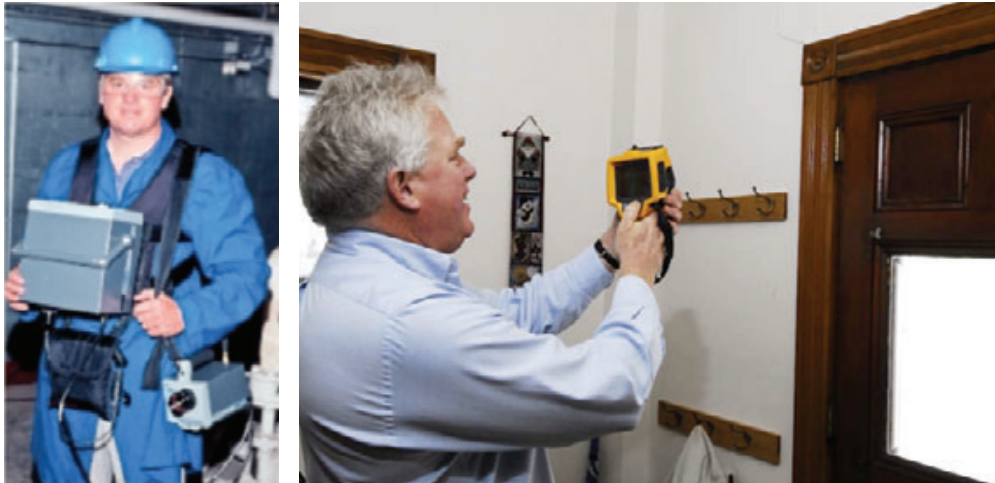
Figure 1. The first commercially available IR cameras weighed anywhere from 10 to 30 pounds and had to be cooled with liquid nitrogen or compressed argon gas (far left). Their modern counterparts are dramatically less expensive and easier to use (left).
