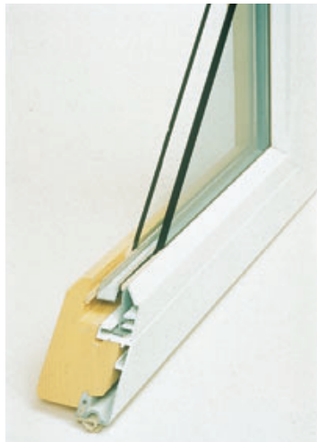
Figure 6. Conductive heat loss around the perimeter of insulated glass units (dark areas in the thermographic image, left) caused by metal edge spacers has led to recent innovations in “warm-edge” nonmetal spacers, such as the PPG Intercept (right).
