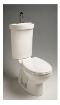
Multitasking Toilet. The Profile Smart Toilet conserves space as well as water, says the manufacturer. Intake water runs through a top-mounted faucet (for hand-washing) before flowing down the sink drain to fill up the tank. Two models are available: the standard-sized Profile Smart 305 and - for universal design applications — the Profile Smart 270, with an elevated (17-inchhigh) elongated seat.
