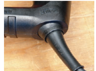
A turret allows the cord to pivot where it exits the tool, improving flexibility and durability.
