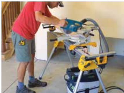
The author's complete rig includes a compact DeWalt stand and a Festool vacuum.
