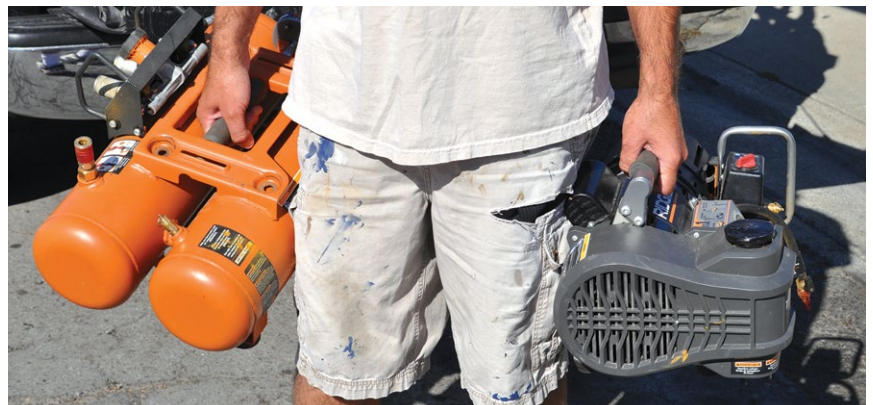
The compressor quickly separates into two parts for easier carrying.
