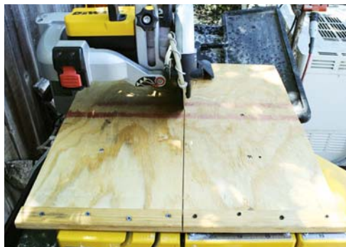
A plywood table clamped to the tile saw's bed (above) and a second water pump with a separate feed line (right) help reduce chipping when cutting glass tile.
