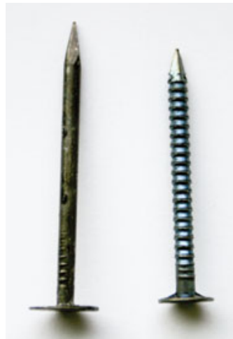
Both the cement-coated smooth-shank drywall nail (far left) and the blued ring-shank drywall nail (left) meet code requirements, but they're more likely to pop than a drywall screw.
