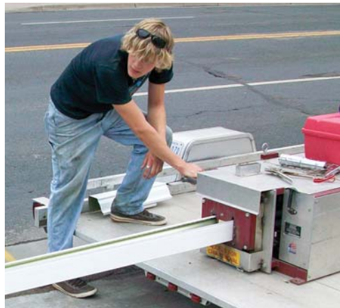
Figure 1. The author's gutter machine, shown here resting on a shop dolly (left), forms a 5-inch K-style profile. For jobs requiring extremely long gutters, he takes the machine to the site (above).
