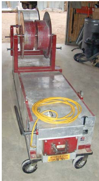
Figure 1. The author's gutter machine, shown here resting on a shop dolly (left), forms a 5-inch K-style profile. For jobs requiring extremely long gutters, he takes the machine to the site (above).
