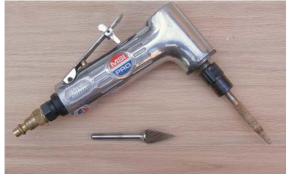
Figure 1. Instead of switching disks, the author switches grinders: He puts 24-grit paper on one tool and uses it for fast stock removal, and 50-grit on the other for precise finishing cuts (left). Curves too tight to grind with a disk are cut with a die grinder equipped with a tapered carbide carving burr or a cone-shaped metalworking burr (above).
