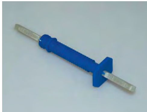
Figure 5. Precast concrete wall panels are formed on a flat casting bed (top). Sandwich panels consist of inner and outer skins of concrete separated by a layer of rigid foam (above); fiber-composite connectors (right) inserted through prepunched holes in the foam during casting hold the inner and outer wythes together.
