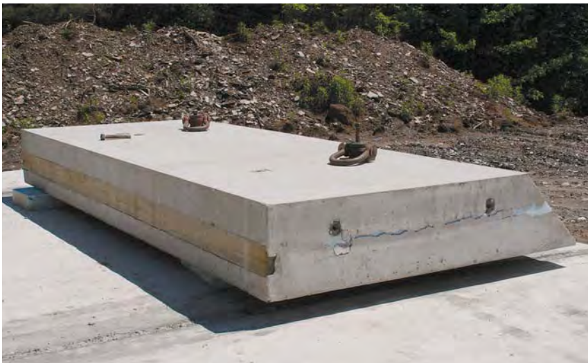
Figure 5. Precast concrete wall panels are formed on a flat casting bed (top). Sandwich panels consist of inner and outer skins of concrete separated by a layer of rigid foam (above); fiber-composite connectors (right) inserted through prepunched holes in the foam during casting hold the inner and outer wythes together.
