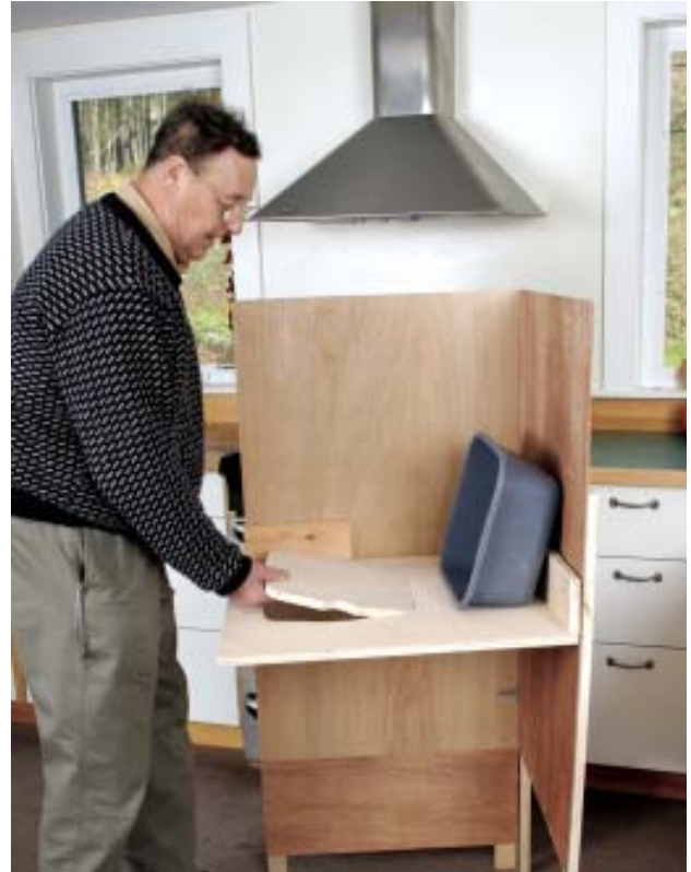
Figure 1. A folding screen fitted with an adjustable countertop helps the author and his clients determine critical countertop dimensions. The plastic dishpan drops into the cutout to approximate knee-space clearance below a sink.
