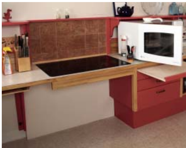
Figure 7. With a recessed glass cooktop, the cook can slide — rather than lift — pots on and off the burners. A combination microwave/convection oven sits at eye level, the perfect height for someone in a wheelchair.
