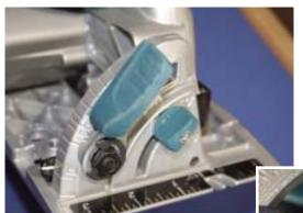
Padded levers make adjusting the bevel and depth settings easier and more comfortable. The small knob is a 45-degree stop; turning it a quarter turn allows the table to swing to a maximum bevel of 51 degrees.
