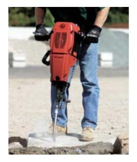
Break Free. Think you need either electricity or a giant tow-behind compressor to run a breaker hammer? Think again. The *Red Hawk* gas-powered breaker has its own two-stroke engine. Weighing in at 50 pounds, the machine can cut clay, concrete, and asphalt; tamp soil and fill; and drive posts and ground rods. A large muffler and a vibration-dampening handle reduce user fatigue. The Red Hawk costs about \$2,200.
