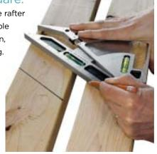
pitches and making plumb and level lines. The device also has an adjustable leg for faster and more accurate repetitive cuts. It comes in a nice nylon case with a roof framing guide and costs \$84.
