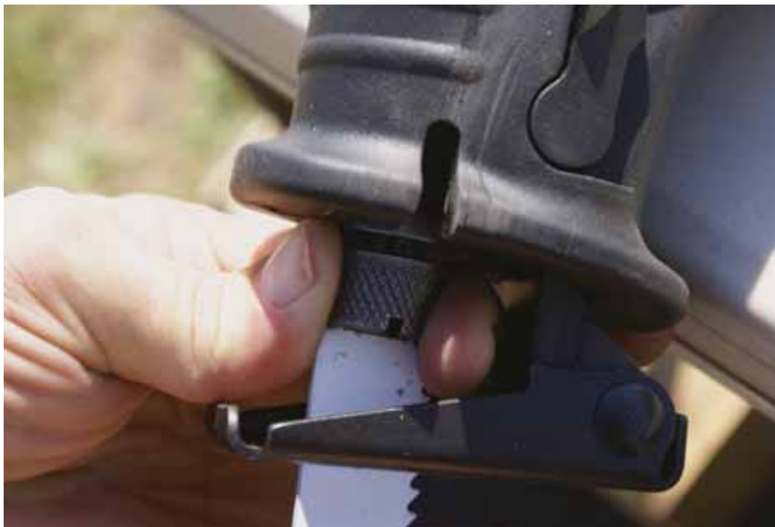
Figure 1. Bosch's blade clamp (top) is the best of the bunch. You simply push the blade in until it clicks. Rotating the metal collar a quarter-turn ejects the blade automatically, reducing the risk of burning your fingers on a hot blade. With no tab or lever, the round collars on the Porter-Cable, DeWalt, and Milwaukee saws (above) were tough to grip.
