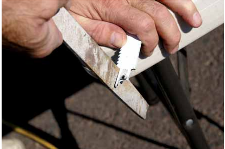
Figure 2. Lenox demolition blades — the author's preference — won't fit in the blade clamps on the Ridgid and Milwaukee saws until the corners where the blade body meets the tang are filed. The process doesn't take long, but it's an inconvenience.
