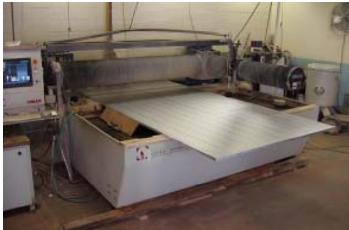
Figure 4. To cut the aluminum bracket components, the author contracted with a local machine shop equipped with an abrasive waterjet. By mixing 80-mesh alluvial garnet with a high-velocity stream of water, the machine was able to slice through the \frac{3}{8} -inch-thick aluminum sheet without overheating or distorting it.
