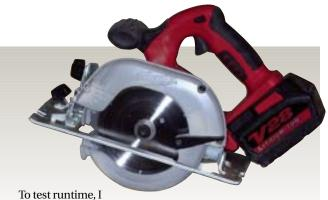
matched it against my 18-volt DeWalt to see how many 2x4s I could crosscut on a single charge. I was able to make 268 cuts with the V28 vs. 122 with the DeWalt. I stopped cutting when I noticed a decrease in performance.
