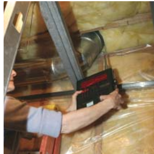
Figure 11. Acoustic treatments should always be tested before drywall is installed. The author uses a tone generator and graphic sound analyzer to measure the decibel level at specific frequencies. If the required STC is not met, she takes additional measures.
