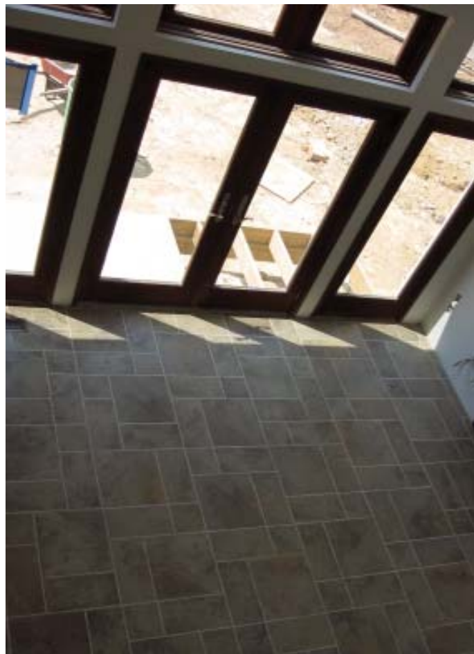
Figure 3. Vertical glazing allows the low-angle winter sun to penetrate deep into a house while mostly excluding the high summer sun, thereby avoiding overheating during the summer (above left and above). Sloped glazing, by contrast, allows year-round penetration and can create uncomfortable overheating during the nonwinter months.
