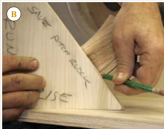
Figure 5. With the volute section laid flat and the easing rising, the pitch block is slid into place and its exact point of contact — the tangent point — marked on the easing (A). Then the pitch block is turned to its complementary angle and scribed across the easing at the tangent point to show the cut line (B). The author screws an auxiliary fence and table to his saw to create a more stable base and a higher continuous fence. A kerf in the base makes it easy to line up the tangent point with the blade. Hot-melt glue secures the pitch block to the volute for support during cutting (C).
