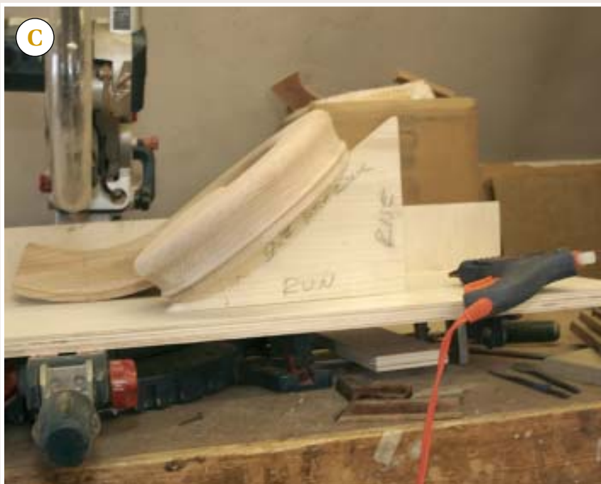
Figure 5. With the volute section laid flat and the easing rising, the pitch block is slid into place and its exact point of contact — the tangent point — marked on the easing (A). Then the pitch block is turned to its complementary angle and scribed across the easing at the tangent point to show the cut line (B). The author screws an auxiliary fence and table to his saw to create a more stable base and a higher continuous fence. A kerf in the base makes it easy to line up the tangent point with the blade. Hot-melt glue secures the pitch block to the volute for support during cutting (C).
