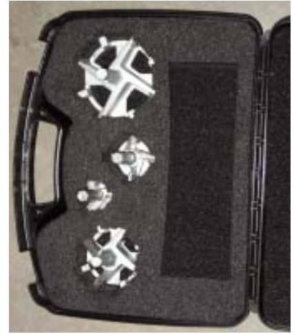
The cutters — which are held in place with screws — cut the pipe as the Pipe Shredder advances into the hub (left). The bits come in a padded case and are sized to fit 1½-, 2-, 3-, and 4-inch pipe (right).
