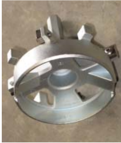
The cutters — which are held in place with screws — cut the pipe as the Pipe Shredder advances into the hub (left). The bits come in a padded case and are sized to fit 1½-, 2-, 3-, and 4-inch pipe (right).
