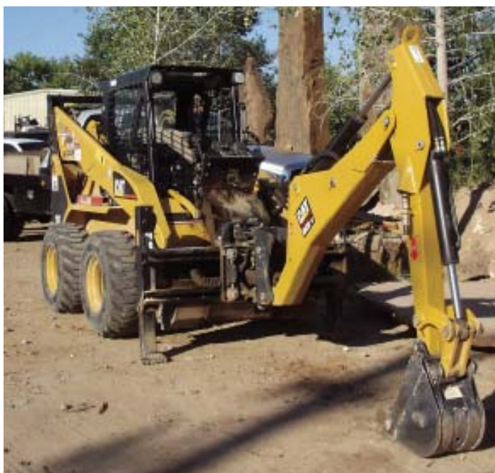
Figure 3. With its short wheelbase and narrow body, a skid-steer loader with a backhoe attachment ($12,000) can fit in places too small for a conventional backhoe. One drawback: Whereas the backhoe is operated from outside the cab, the skid steer itself is controlled from inside — an arrangement that can lead to a lot of clambering in and out of the cab.
