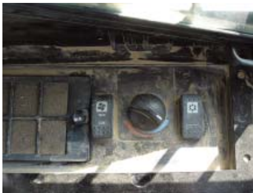
Figure 2. Considered a necessity by the author, a closed cab with air conditioning makes operators more efficient and increases safety by eliminating extreme heat as a source of fatigue. It also helps with employee retention: An uncomfortable operator may be lured away by another employer with air-conditioned equipment.
