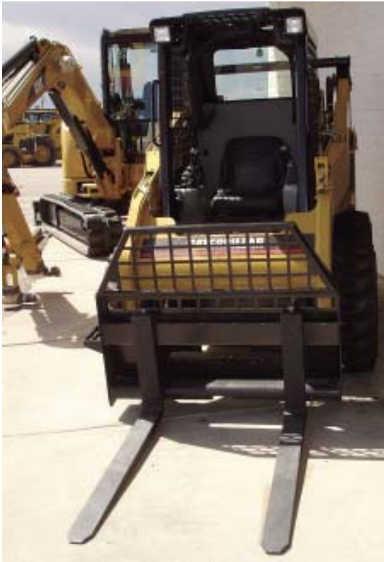
Figure 4. Pallet forks — which cost about $1,000 — are one of the most valuable attachments, allowing GCs to unload trucks and move heavy materials quickly and effortlessly.
