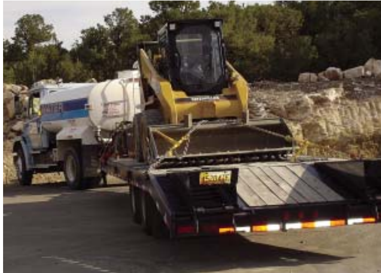
Figure 8. Moving a skid steer requires a sturdy trailer rated for the machine's weight as well as for any additional attachments carried along. The machine should be secured to the trailer at four points with grade 70 \frac{5}{16} -inch chain. Nylon straps are insufficient.
