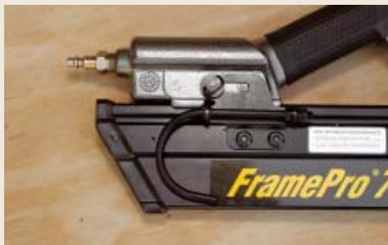
Figure 1. Paslode's gun (top) has a beefy spring-loaded rafter hook that folds out for use. DeWalt's hook (center) is made from plastic; it stows pretty well but is still somewhat obtrusive. Senco's hook (bottom) folds neatly out of the way when the gun is in use.
