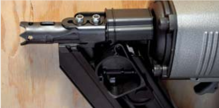
Figure 2. It takes a small wrench to adjust the old-style depth-of-drive mechanism on the FramePro 601 (above). The Paslode (right) uses an Allen wrench, which stores in the back of the magazine.
