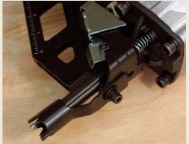
Figure 2. It takes a small wrench to adjust the old-style depth-of-drive mechanism on the FramePro 601 (above). The Paslode (right) uses an Allen wrench, which stores in the back of the magazine.
