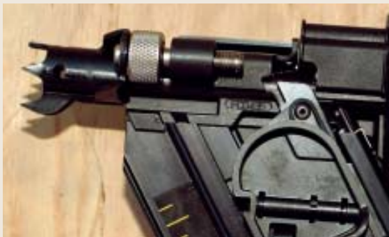
Figure 3. The Makita (top) and Hitachi's NR 90AD (center) have indexed thumb-wheels just below the trigger to control depth of drive. The thumb-wheel that controls depth of drive on the Senco FramePro 701XP (bottom) is cleanly integrated into the nose.
