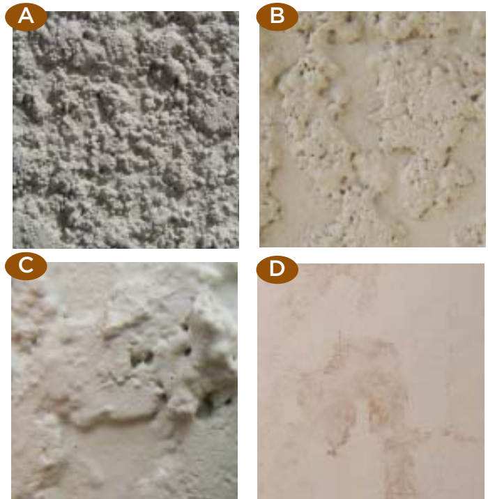
Figure 9. Paints and coatings are not highly effective at spanning cracks and pinholes in a rough stucco coating. Ordinary paint (A), a 3-mil high-build coating (B), and a 10-mil elastomeric coating (C) all leave pinholes that can be seen under magnification. Thick elastomeric coatings over stucco can also be prone to blistering (D).
