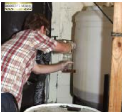
Converting used vegetable oil into biodiesel is a fairly simple process: The oil is mixed with catalysts and heated in a tank (above). The finished product (right) is amber brown and chemically similar to No. 2 heating oil.
