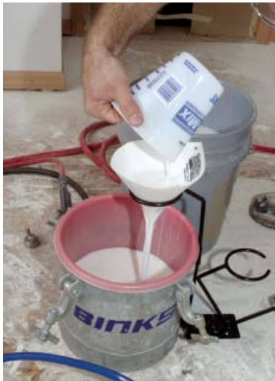
Figure 4. In storage, solids in the waterborne lacquer settle quickly to the bottom. Even after a thorough stirring, lumps may linger and cause gun clogs if delivered from the pressure pot. Straining through a 20-cent paper filter eliminates most of that risk.
