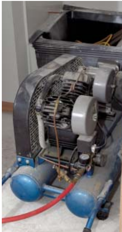
Figure 3. The author's spray equipment includes a compressor (left) that he uses far more commonly to drive nail guns than to power the pressure pot. Any compressor capable of delivering 80 psi is adequate for painting. The pressure pot itself (above) consists of a 2.8-gallon reservoir and an airtight lid equipped with air and fluid outlets, each independently regulated. The pressure pot allows a high degree of control over air and fluid delivery to the gun, which has a direct effect on the quality of the spray job.
