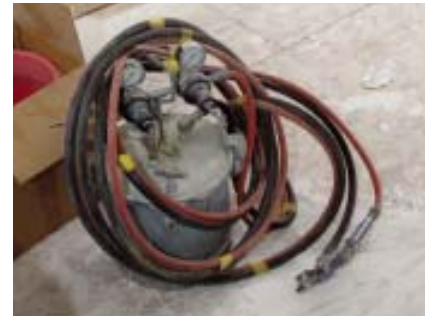
Figure 3. The author's spray equipment includes a compressor (left) that he uses far more commonly to drive nail guns than to power the pressure pot. Any compressor capable of delivering 80 psi is adequate for painting. The pressure pot itself (above) consists of a 2.8-gallon reservoir and an airtight lid equipped with air and fluid outlets, each independently regulated. The pressure pot allows a high degree of control over air and fluid delivery to the gun, which has a direct effect on the quality of the spray job.
