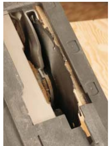
Figure 4. A zero-clearance insert and the guide itself work together to ensure a splinter-free cut on both sides of the blade. The insert snaps into the bottom of the sled and is cut the first time the saw is lowered. The manufacturer provides four inserts — two that work with the guide and two for freehand cutting. The extra inserts allow you to use a variety of blade thicknesses.
