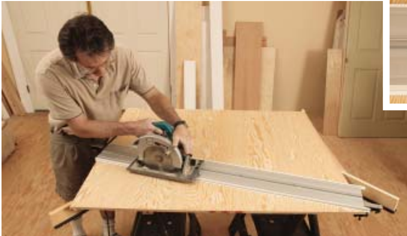
Figure 3. Made from two aluminum sections, the EZ Smart Guide provides a simple and accurate way to trim door bottoms and cut panel products (above). Guide sections are joined with tight-tolerance splines and set screws (right, top); clamps can be placed anywhere along the aluminum extrusion (right, bottom).
