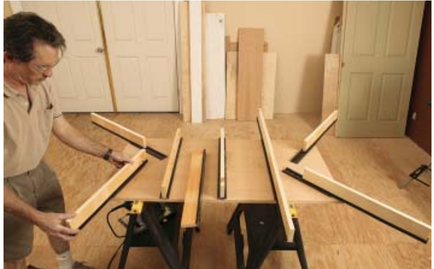
Figure 2. The instructions suggest positioning the end supports so they butt end to end. However, by offsetting them slightly, all four end cleats can remain on the table when the table is at its smallest, making transport and setup easier.
