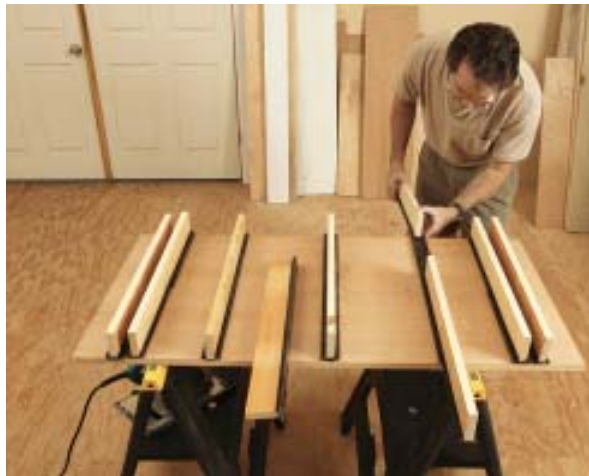
Figure 2. The instructions suggest positioning the end supports so they butt end to end. However, by offsetting them slightly, all four end cleats can remain on the table when the table is at its smallest, making transport and setup easier.
