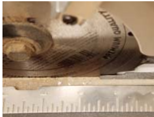
Figure 3. Made from two aluminum sections, the EZ Smart Guide provides a simple and accurate way to trim door bottoms and cut panel products (above). Guide sections are joined with tight-tolerance splines and set screws (right, top); clamps can be placed anywhere along the aluminum extrusion (right, bottom).
