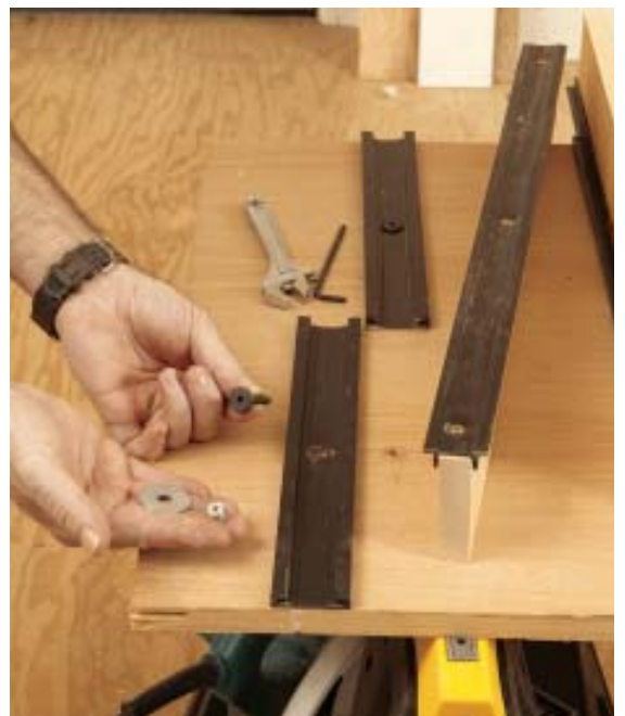
Figure 1. Thanks to sliding supports, the Smart Table can support a full sheet of plywood (top) or a large face frame (above) and then collapse to a 2-foot-by-4-foot size for transport and storage. The plastic slides attach to 1-by support cleats and ride in corresponding plastic tracks; since the end cleats are secured with a single bolt, they can be positioned as needed (right).
