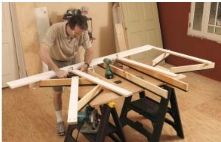
Figure 1. Thanks to sliding supports, the Smart Table can support a full sheet of plywood (top) or a large face frame (above) and then collapse to a 2-foot-by-4-foot size for transport and storage. The plastic slides attach to 1-by support cleats and ride in corresponding plastic tracks; since the end cleats are secured with a single bolt, they can be positioned as needed (right).
