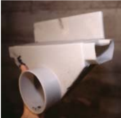
Figure 4. An adapter (above) connects the uniquely shaped WaterGuard footing drain to a length of 4-inch PVC pipe that runs into the sump basket. Workers use a jigsaw to remove the knockout in the sump basket (above right); then they level the basket and backfill around it with washed stone (right).
