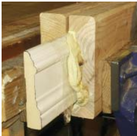
Figure 2. Once the prepared blank has been “battered” with a hard-setting filler, the molding is pressed into place with a vise to form a perfectly detailed negative pattern.
