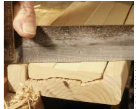
Figure 1. The basic pattern of each molding is roughed out with a table saw and cleaned up with a chisel. A sample piece of molding should fit the opening with 1/16 inch or so of clearance.
